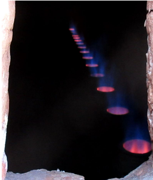
Figure 9: Premix Zone Firing (Manual Operation)
